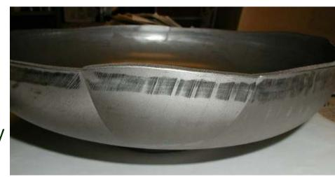
Metal bending requires dislocation motion on slip systems Nb is a BCC metal like Fe; not FCC like Al or Cu, or HCP like Ti; Need geometry of crystal orientation, slip planes & directions
